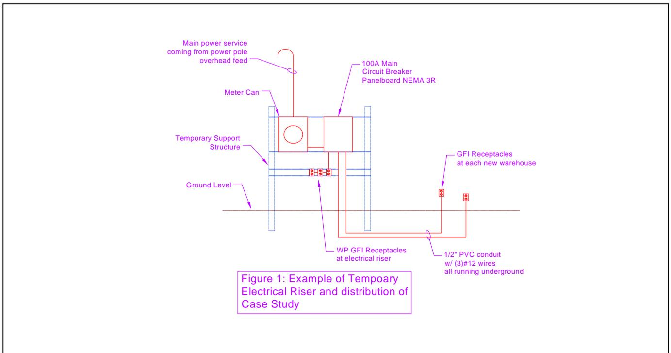
**Figure 1: Example of Temporary Electrical Riser and Distribution for Case Study**
